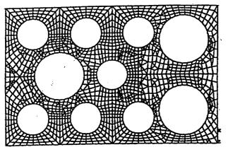
Linear elastic finite plate element model
