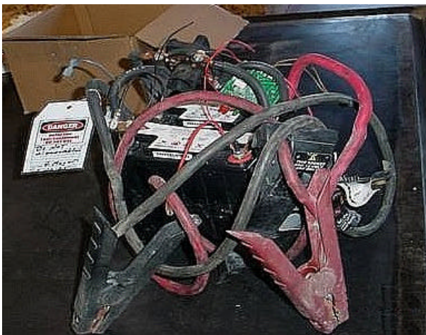
Figure 1. The damaged battery booster after the explosion
