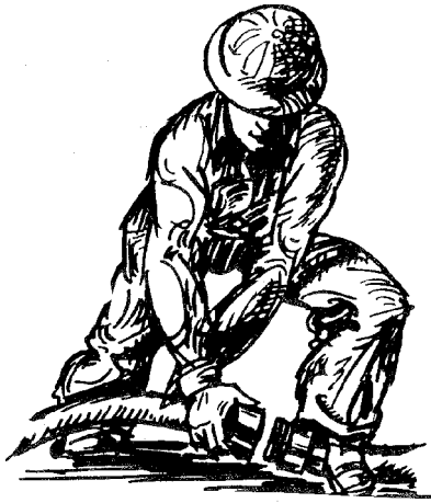
Figure 4. One man connecting fire hose.
