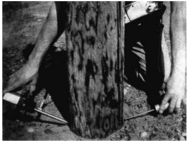
Figure 3. The Pol-Tek sonic tester.
