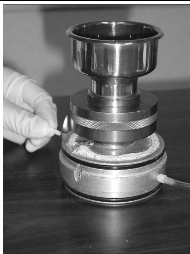
Figure 7.1-1. Procedure to flame sterilize the Millipore Hydrosol ® field filtration unit.
