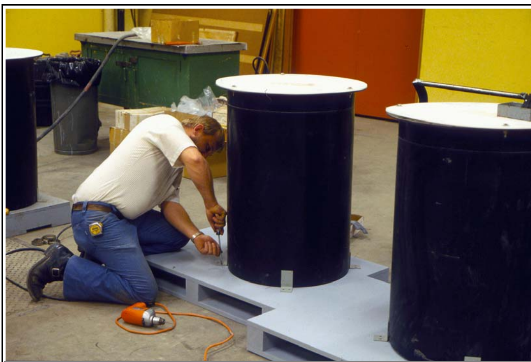
Figure 9a.—Sediment-water simulation microcosms under construction.
