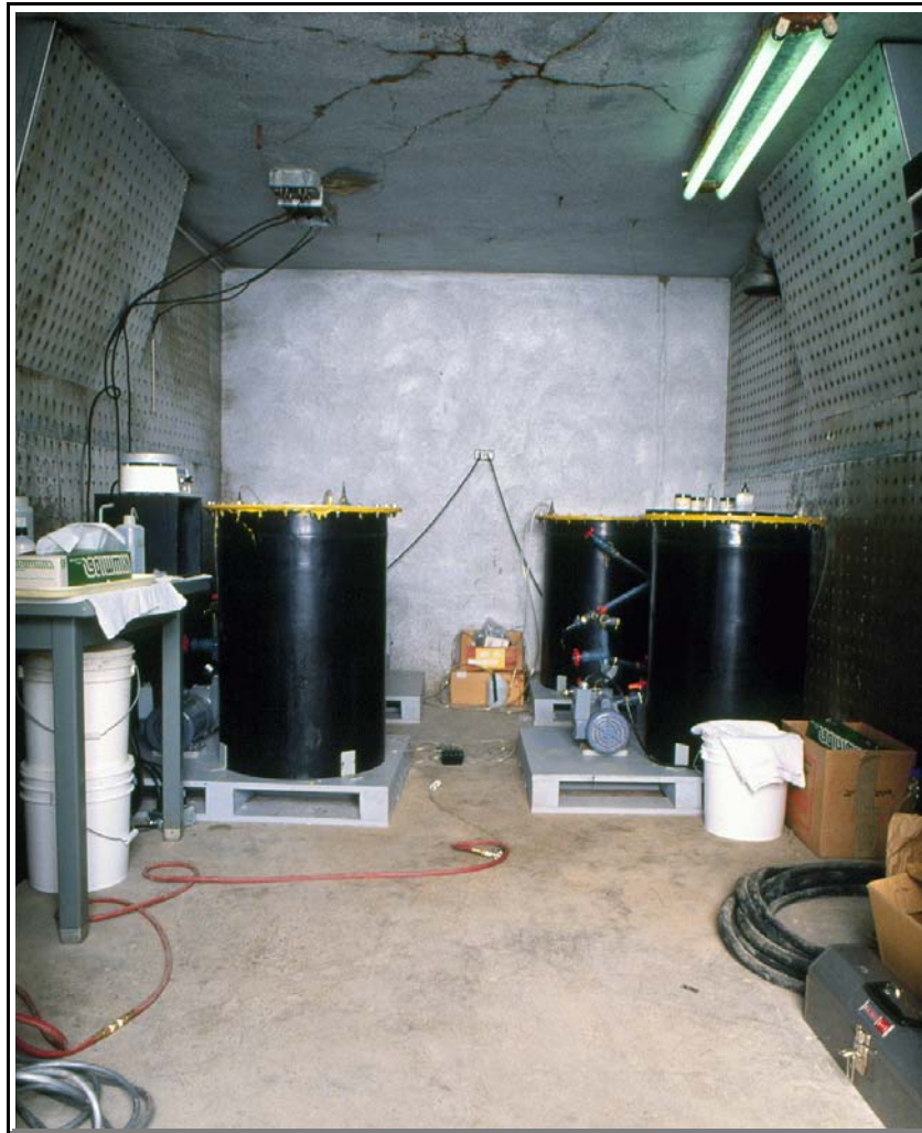
Figure 11.—View of the sediment-water microcosms located in an old calorimeter room at the Bureau of Reclamation's Denver facility. The pumps and sidearm plumbing were removed for sampling under anaerobic conditions.
