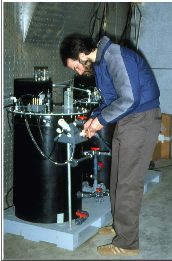
Figure 9b.—Completed simulation tank with circulation sidearm and instrumentation. These items were removed for the anaerobic portion of the simulation.
