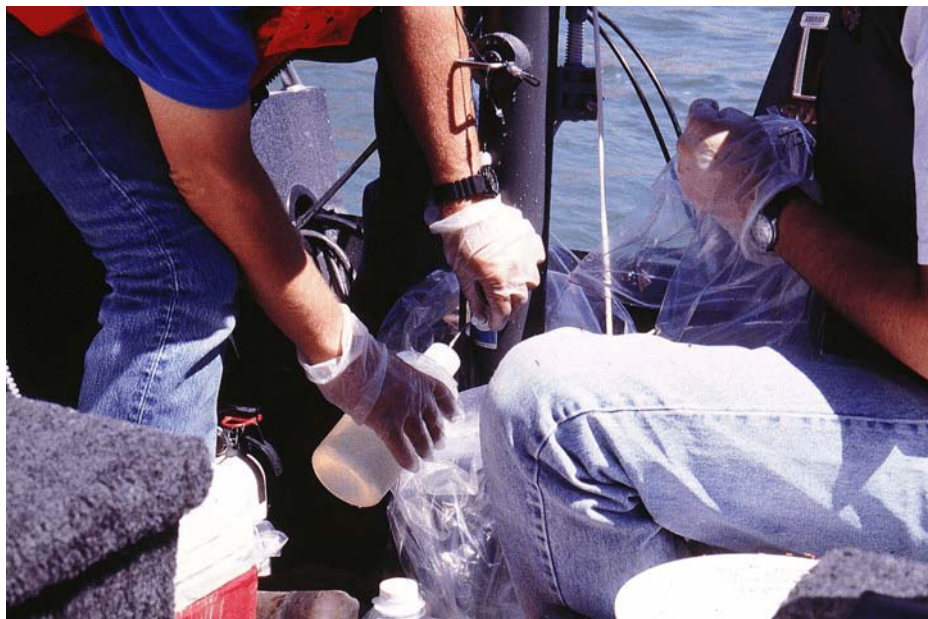
Figure 3.— Clean-hands/dirty-hands sampling of water for low concentrations of Hg and Me-Hg. The clean-hands (person, on the left) touches the Teflon sample bottle. The dirty-hands person (right) only handles the plastic bag which is sealed before shipping.
