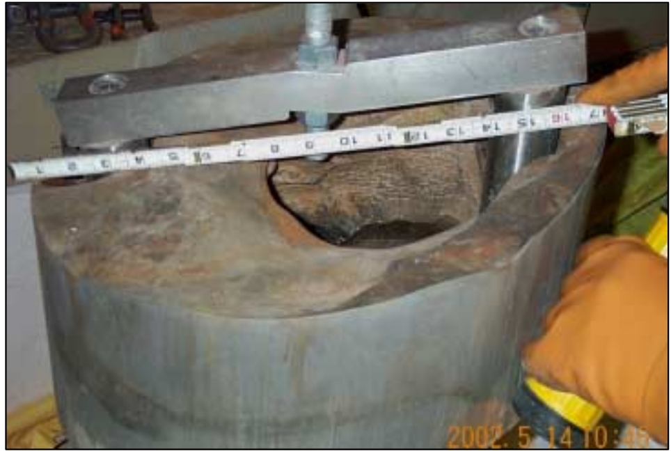
Nozzle #3 Area Cut Away From Reactor Head
