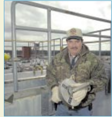
Savannah River Site (SRS) facility personnel developed a simple modification which incorporates the valve wrench/handle into the valve port cover to allow remote valve operations during the transfer of liquid wastes between tanks at the SRS High-Level Waste Tank Farm. Their innovation meant that the large valve/jumper box area could be "rolled back" to a contamination-free area resulting in reduced waste.
