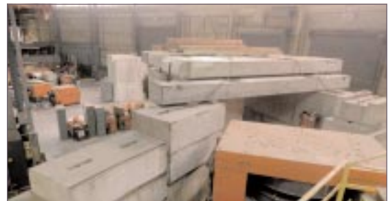
After the closure of the Lawrence Berkeley National Laboratory’s Bevalac facility, 19,000 metric tons of reinforced, high-density concrete shielding blocks were no longer needed. More than one-third of them were reused at the Brookhaven National Laboratory as shielding. This is equivalent to sixty rail locomotives.
