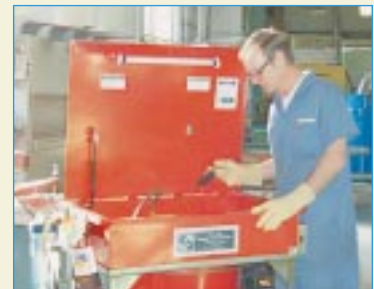
Hanford Site machinists utilize a parts washer that continually filters and cleans machine solvent. The washer extends the life of the solvent and reduces the procurement of new solvent and the generation of waste.
