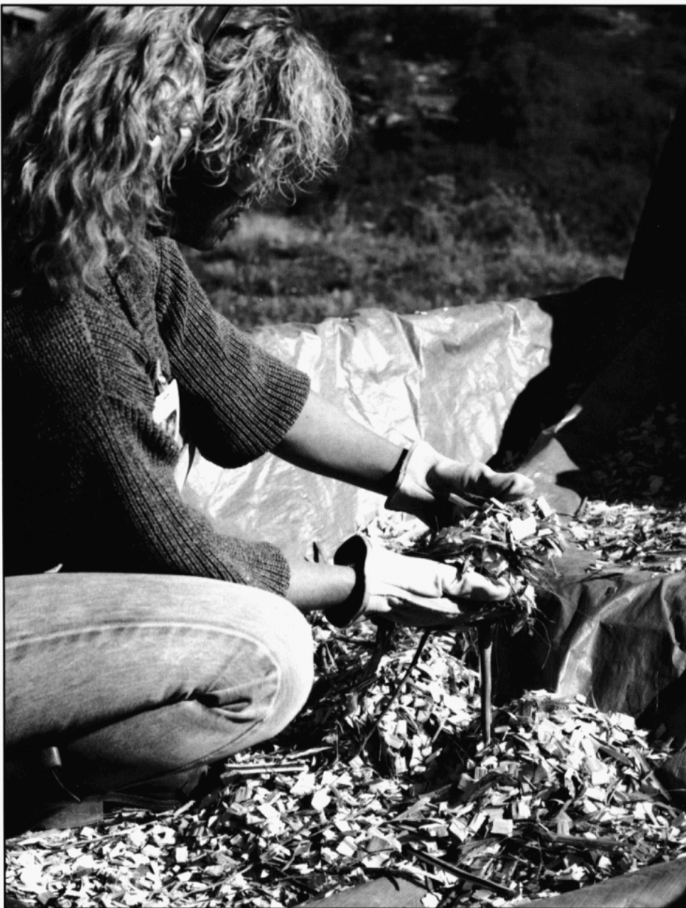
An NREL researcher prepares wood chips for fuel conversion. These chips will be ground up, pretreated, and used in the NREL simultaneous saccharification and fermentation (SSF) process.
