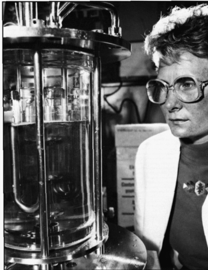
The SSF method of ethanol production (the SSF process vessel is shown here) increases yields, decreases process time, and lowers production costs because the saccharification and fermentation steps take place simultaneously.
