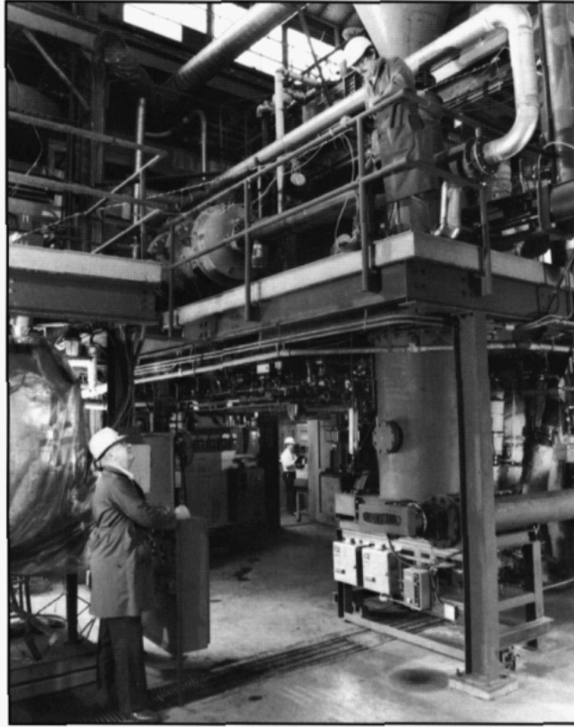
The Battelle high-throughput biomass gasification process is one of the most promising methanol production technologies being investigated by the BSD program.
