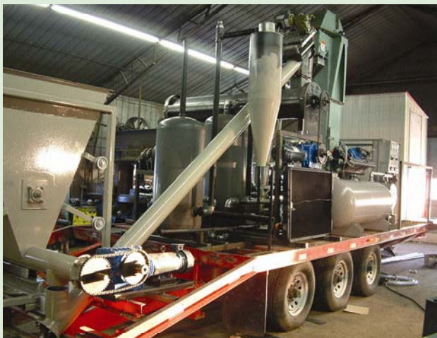
Figure S-1.1 A Small scale portable reactor for liquid fuel production by distributed fast pyrolysis.
