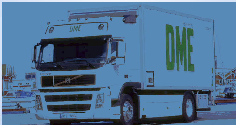
Figure 4.3 Volvo’s 2nd Generation Heavy-Duty prototype DME vehicle, developed under the EU-sponsored “AFFORHD” (Alternative Fuel For Heavy-Duty) project in 2005.
