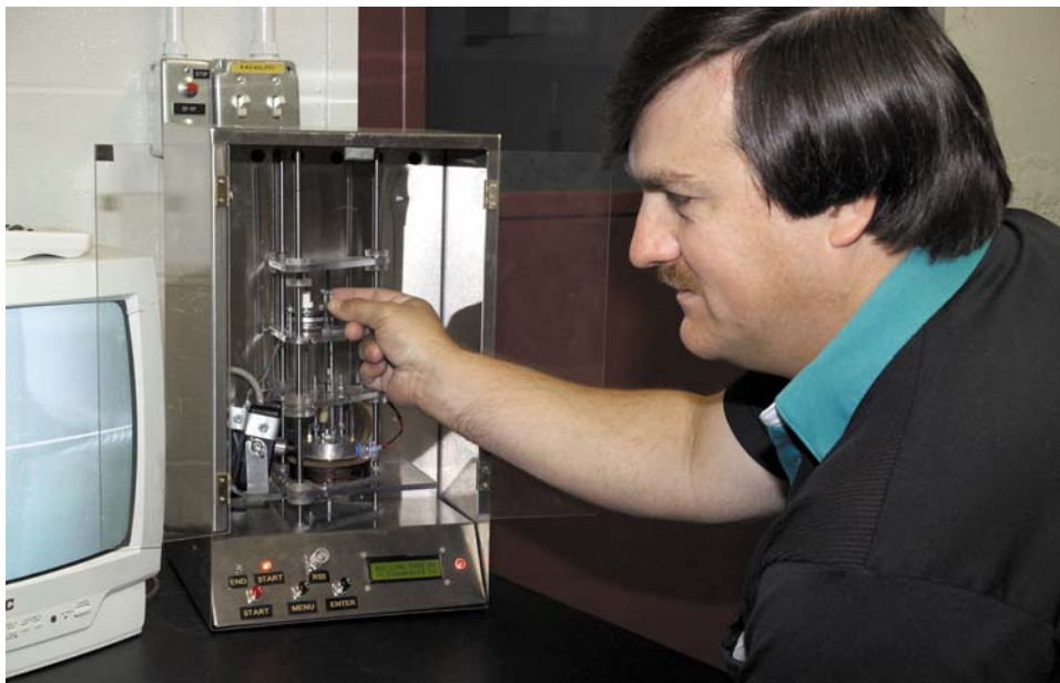
KCP CLEANING TECHNOLOGY: Mark Benkovich, KCP staff engineer, positions solvent that has been used to clean a part in the MicroSolventEvaporator™. The MicroSolventEvaporator™ quickly evaporates the solvent, leaving only extracted residue on a clean reference substrate, ready to be tested for organic contaminants in the MESERAN™ Analyzer.
