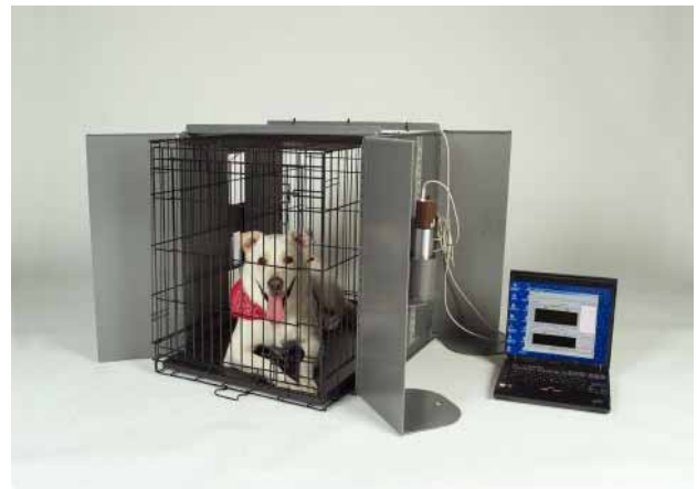
ANIMAL PORTAL MONITOR: Pet portal system designed by Bechtel Nevada scientists allows radiation technicians to survey family pets faster without having to handle the animals
