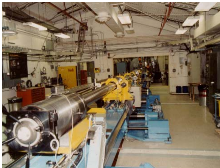
The JASPER gun is an approximately 90 foot long, two stage gun.
