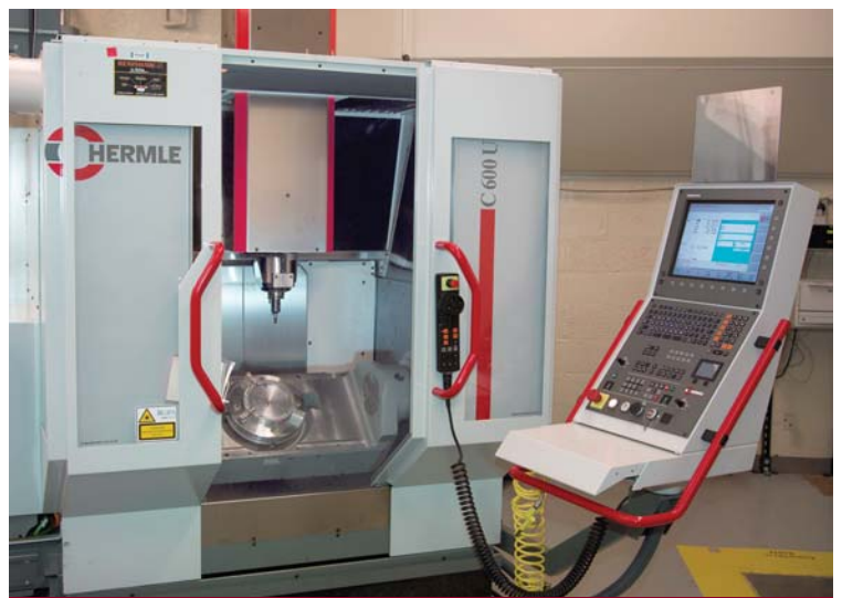
NNSA LEADS TECHNICAL TRAINING: An export controlled 5-Axis machine tool useful for making parts for commercial and weapons use, featured in a training session at the Kansas City Plant.
