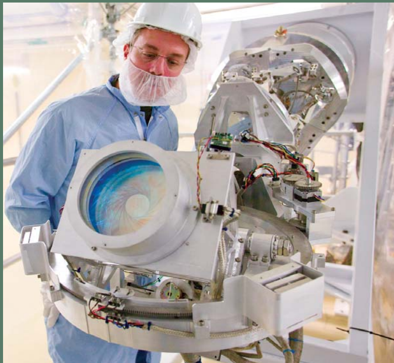
NIF OPTICS CHECKER: A National Ignition Facility technician examines a damage inspection instrument that is used to assess the optics in the target chamber.
