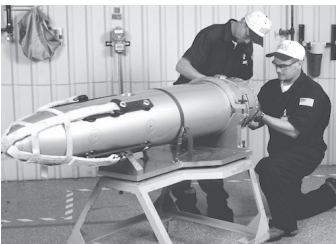
Two workers at the Pantex Site Office that are working on a B 61 tail section.
