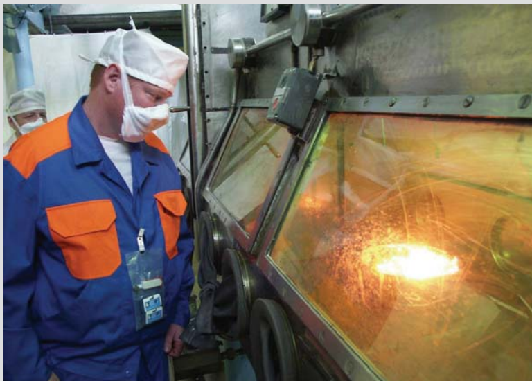
DOWNBLENDING EXPERTISE: A U.S. expert observes as highly enriched uranium metal is converted to oxide.
