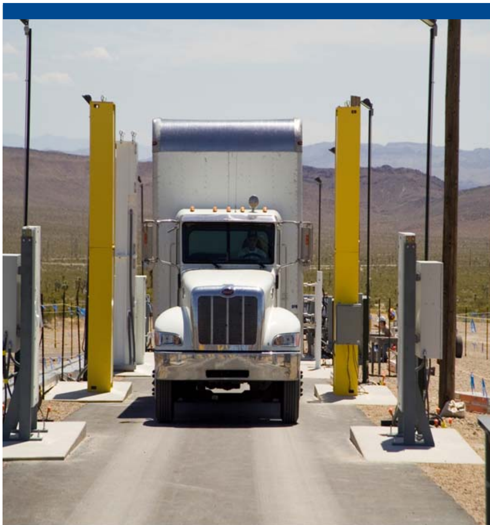
CUTTING EDGE TESTING: A truck drives between Advanced Spectroscopic Portals during testing at the Nevada Test Site.
