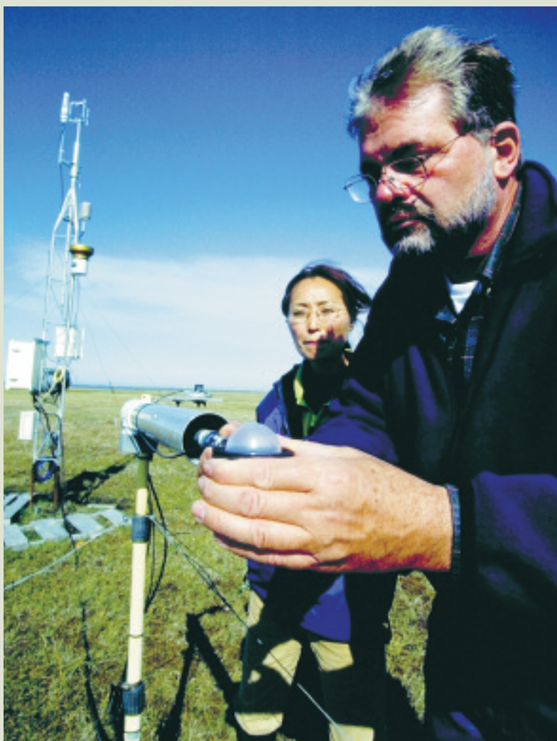
Monitoring Carbon Flows. Scientists near Pt. Barrow, Alaska, check instruments that measure fluxes of carbon to and from the atmosphere. Source: Gary Braasch.
