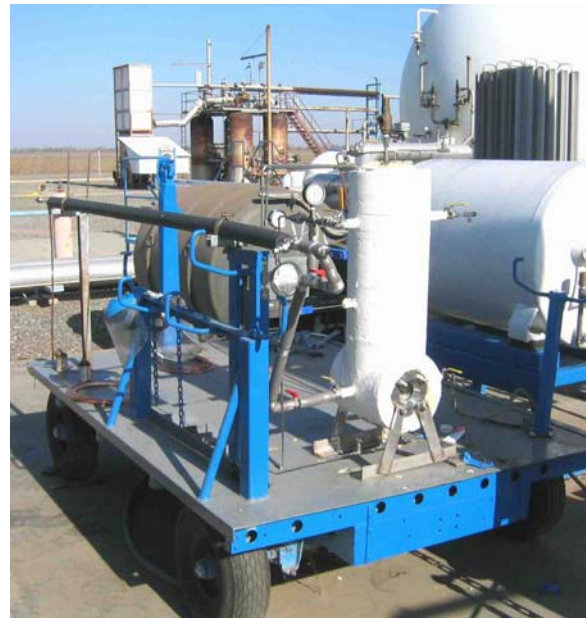
Figure 1. CryoSystems International LNG odorization test fixture.
