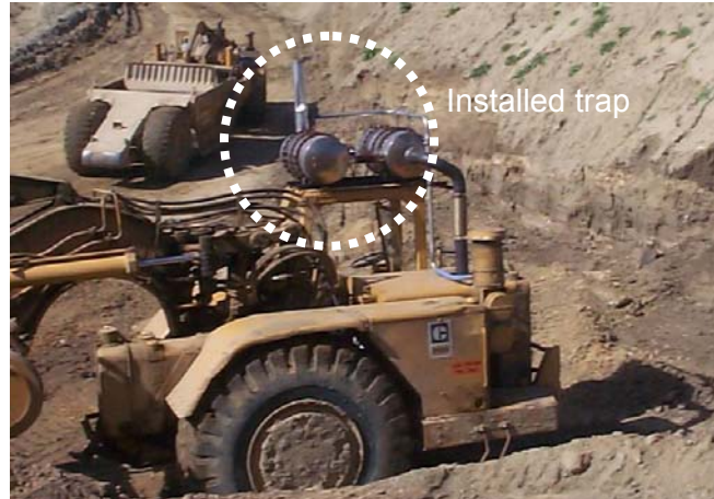
Figure 7: Installed Particulate Trap on Heavy-Duty Construction Equipment
