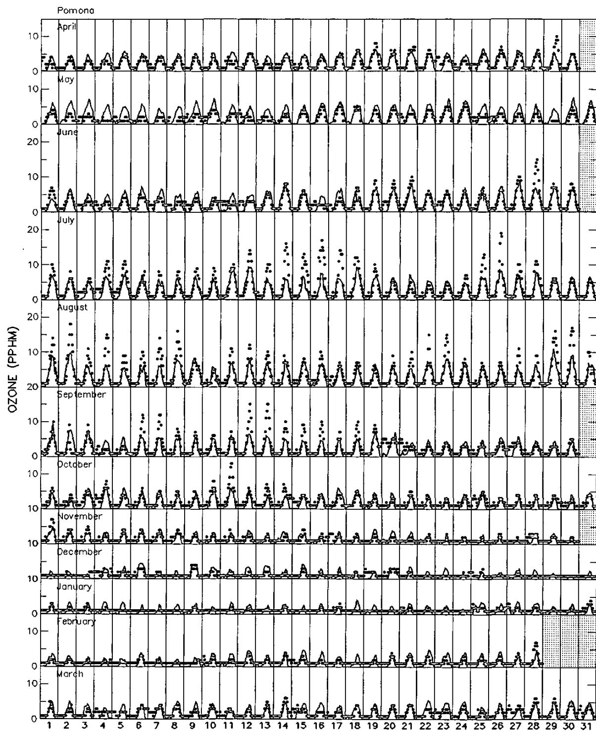
Figure V-7d. Comparison between UAM-TOX predicted (solid line) and measured (points) 1-hour average ozone concentrations (pphm) at Pomona (April 1, 1998 – March 31, 1999).
