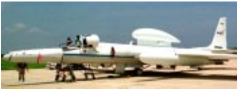
NASA aircraft used in CAMEX-3 were the ER-2, a single-seat, high-altitude research jet (top) and the DC-8 Airborne Laboratory (below), a converted jetliner with room for several scientists and their equipment (bottom). (NASA)
