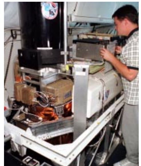
The Lidar Atmospheric Sensing Experiment (LASE) made the first lidar measurements of water vapor inside the eye of a hurricane. LASE measured profiles of aerosols (upper) and water vapor (lower) when the DC-8 flew through the eye of Hurricane Bonnie on Aug. 26, 1998, just before the storm hit the east coast of the U.S. A broken cloud field was visually observed in Bonnie’s eye. LASE measurements showed this eye to be quite large and revealed the precise altitudes of clouds within the eye. LASE also measured the vertical distribution of water vapor inside the eye of Bonnie during brief cloud free periods. LASE was mounted in the DC-8 Airborne Laboratory. (NASA)
