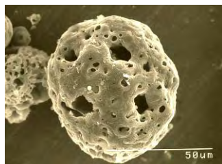
Figure 3-4. Scanning Electron Micrograph of a Spheroidal Carbonaceous Particle (SCP). Photo: Neil Rose.
