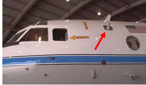
Figure 11. P3 With TAMDAR Installed
