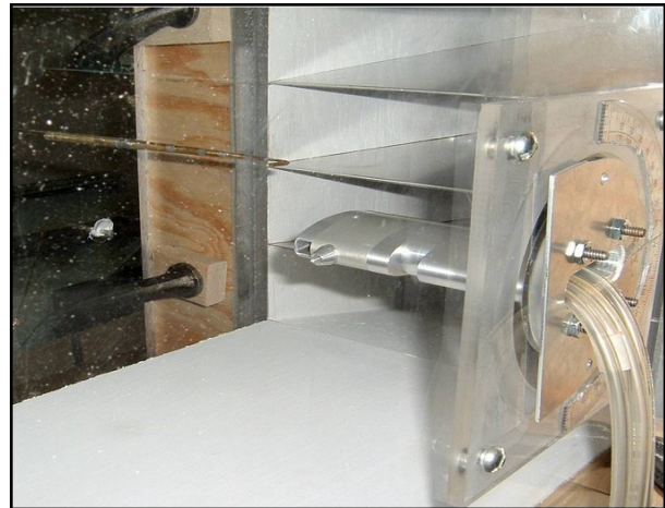
Figure 3. TAMDAR mounted in the UND Wind Tunnel Test Section
