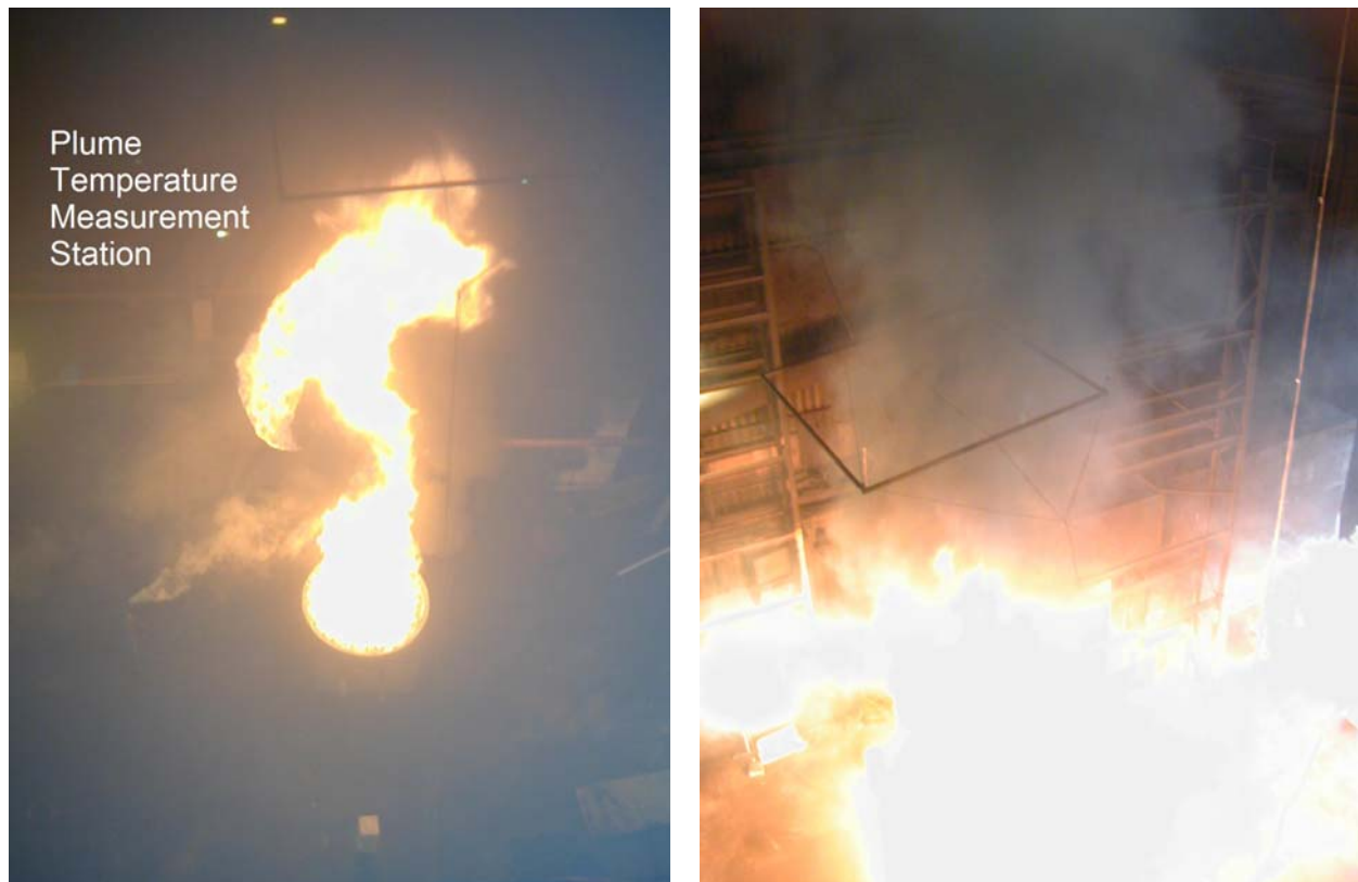
Figure A-21. Photographs of fire plumes in ICFMP BE #2. Courtesy Simo Hostikka, VTT Building and Transport, Espoo, Finland.
