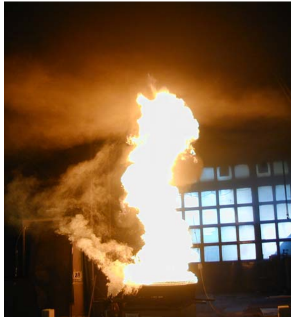
Figure A-25: Photographs of heptane pan fires, ICFMP BE #2, Case 2. Courtesy, Simo Hostikka, VTT Building and Transport, Espoo, Finland.
