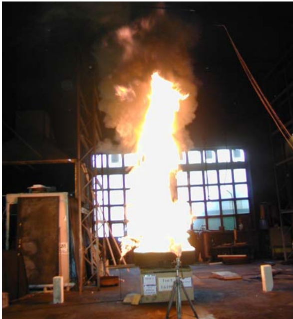
Figure A-25: Photographs of heptane pan fires, ICFMP BE #2, Case 2. Courtesy, Simo Hostikka, VTT Building and Transport, Espoo, Finland.
