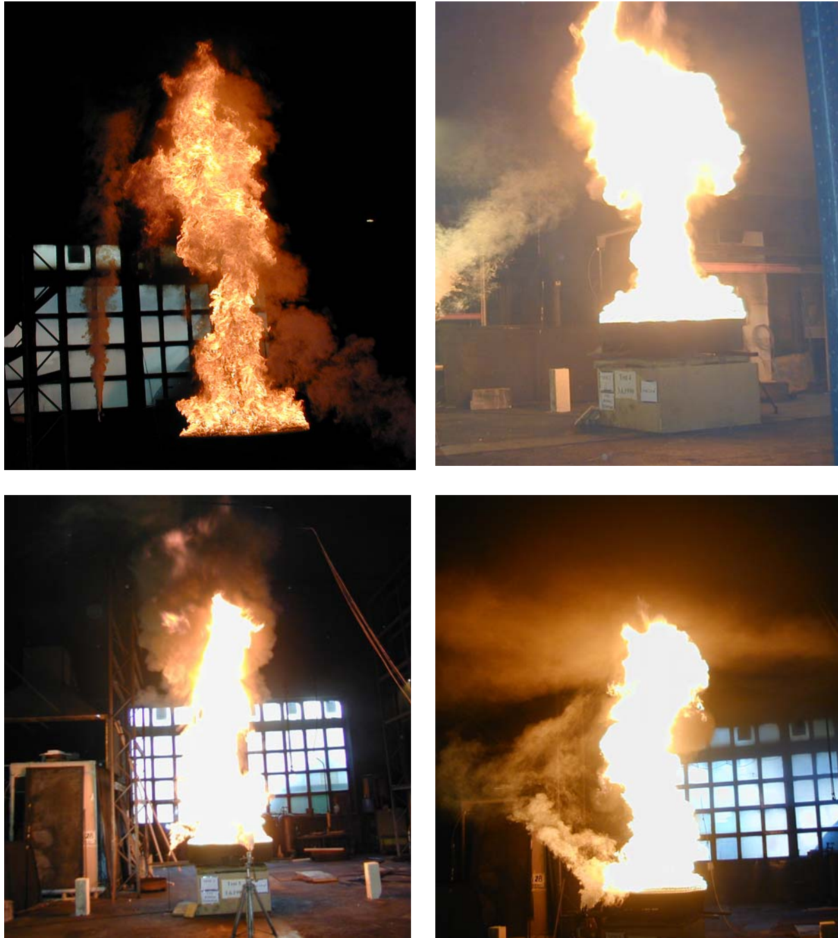
Figure A-18. Photographs of heptane pan fires, ICFMP BE #2, Case 2. Courtesy, Simo Hostikka, VTT Building and Transport, Espoo, Finland.
