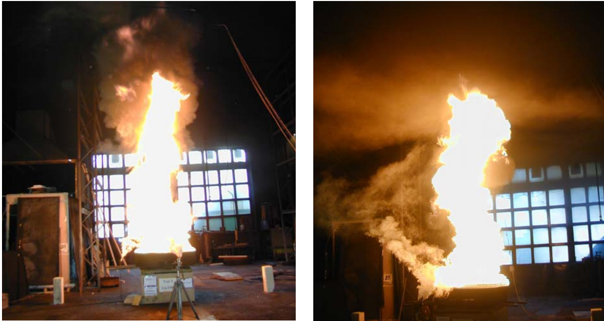
Figure A-20: Photographs of heptane pan fires, ICFMP BE #2, Case 2. Courtesy, Simo Hostikka, VTT Building and Transport, Espoo, Finland.
