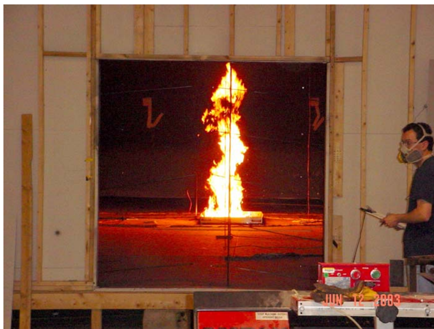
Figure A-21: Photograph and simulation of ICFMP BE #3, Test 3, as seen through the 2 m by 2 m doorway. Photo courtesy of Francisco Joglar, SAIC.
