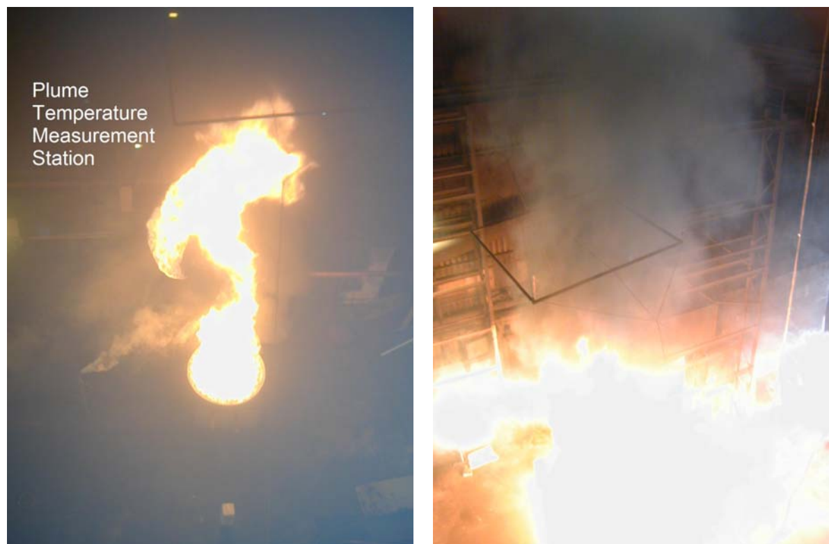
Figure A-15: Fire plumes in ICFMP BE #2. Courtesy Simo Hostikka, VTT Building and Transport, Espoo, Finland.
