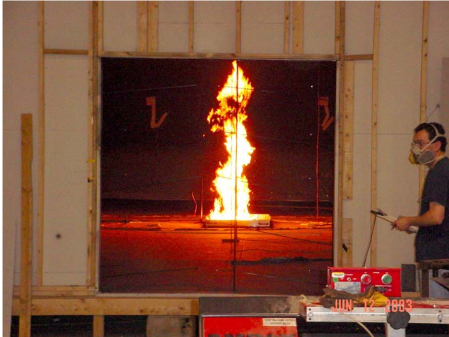
Figure A-13: Photograph and simulation of ICFMP BE #3, Test 3, as seen through the 2 m by 2 m doorway. Photo courtesy of Francisco Joglar, SAIC.
