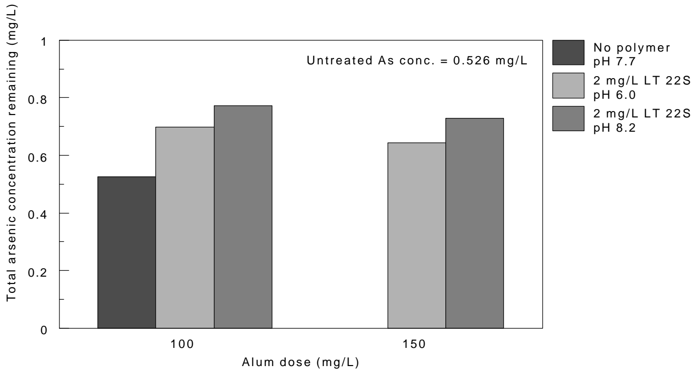
Figure A-7. Total arsenic remaining in the supernatant after alum precipitation for reverse osmosis (A) concentrate
