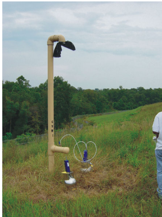
Landfill Gas Sampling with Duplicate Sampling and Ambient Air Sampling at a Passive Vent
