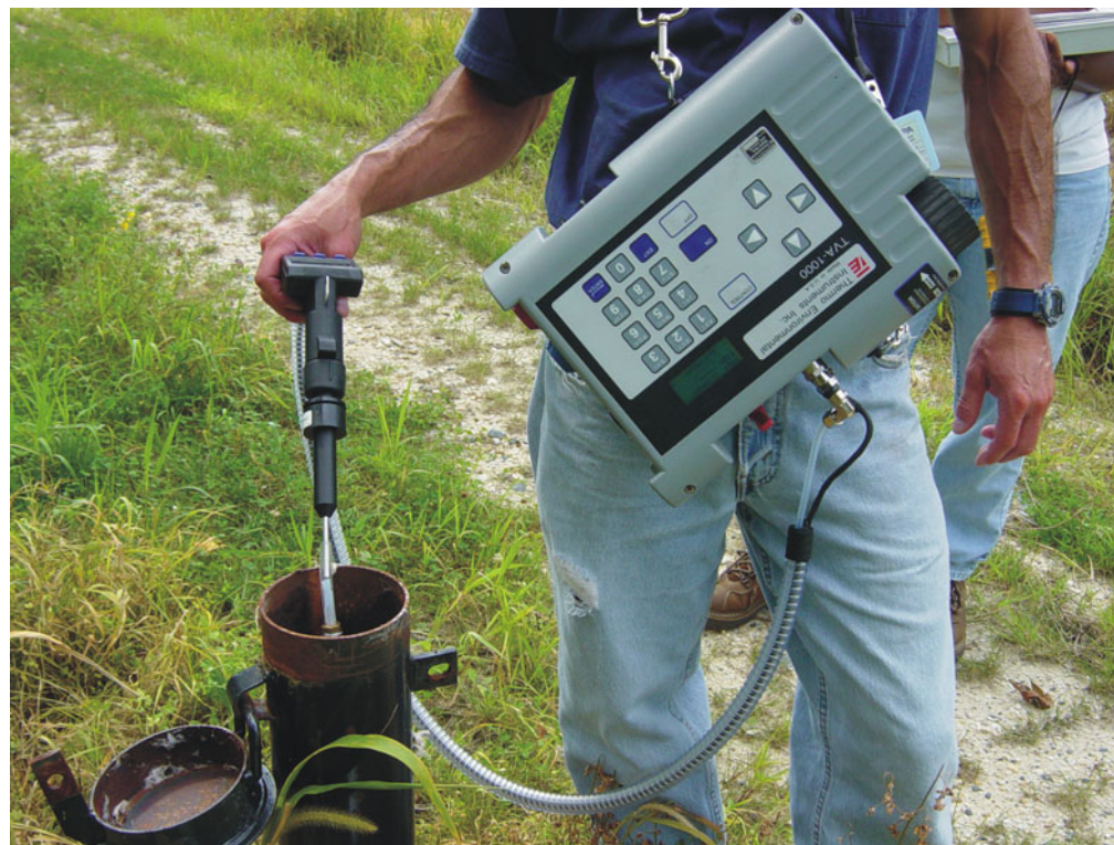
Landfill Gas Screening of a Perimeter Gas Monitoring Probe
