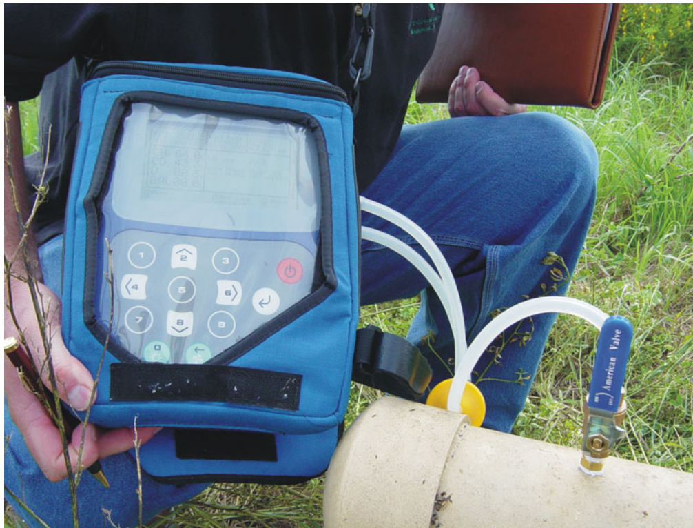
Landfill Gas Screening at a Passive Vent
