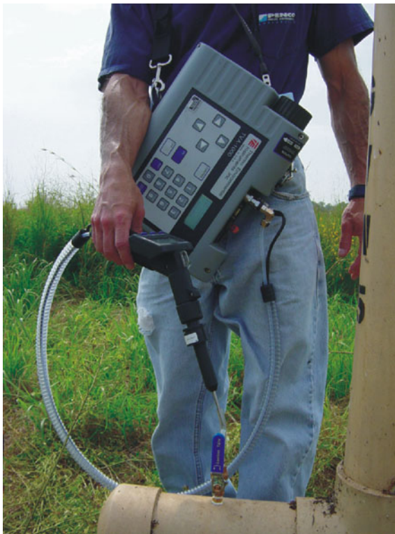
Landfill Gas Screening at a Passive Vent
