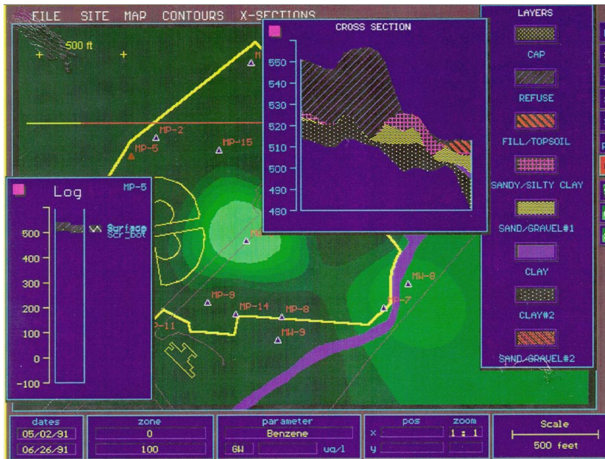
Figure 6. GEOS computer screen showing organic contaminant plume in relation to subsurface stratigraphy (see text for discussion).
