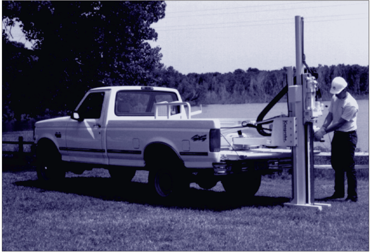
Figure 4. Hydraulic or vibratory direct-push rigs can be installed on vans, small trucks, all-terrain vehicles, or trailers and allow collection of continuous soil cores and depth-specific ground-water samples for detailed subsurface mapping if contaminants are generally confined to depths of less than 15 meters. (Photo courtesy of Geoprobe Systems.)
