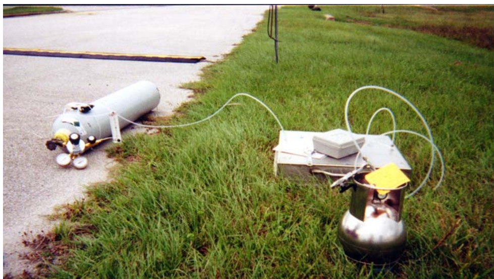
Figure 4-7. Surface Emissions Testing at Launch Complex 34
