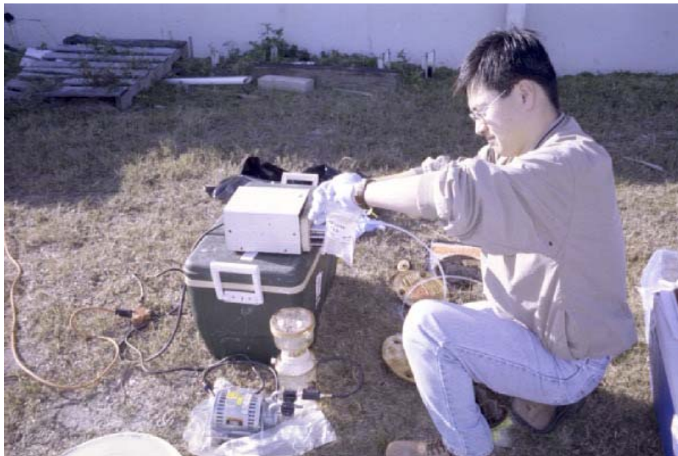
Figure 4-6. Collecting and Processing Groundwater Samples for Microbiological Analysis
