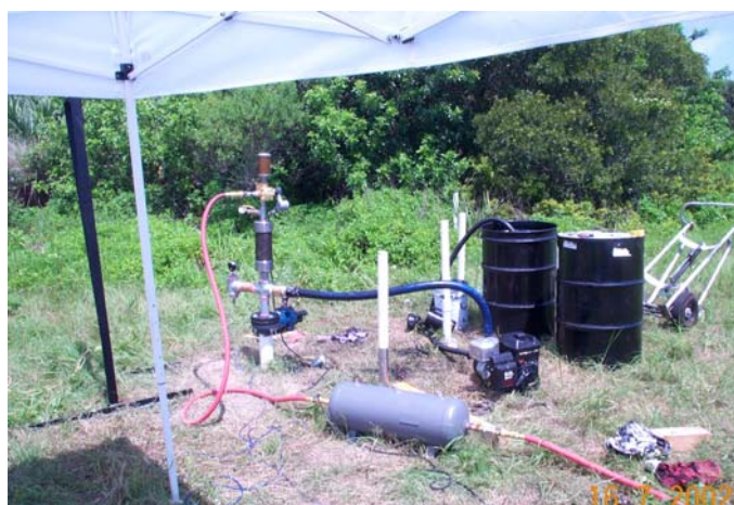
Figure 3-2. Field Injection Test Setup with PPT Injection Technique
