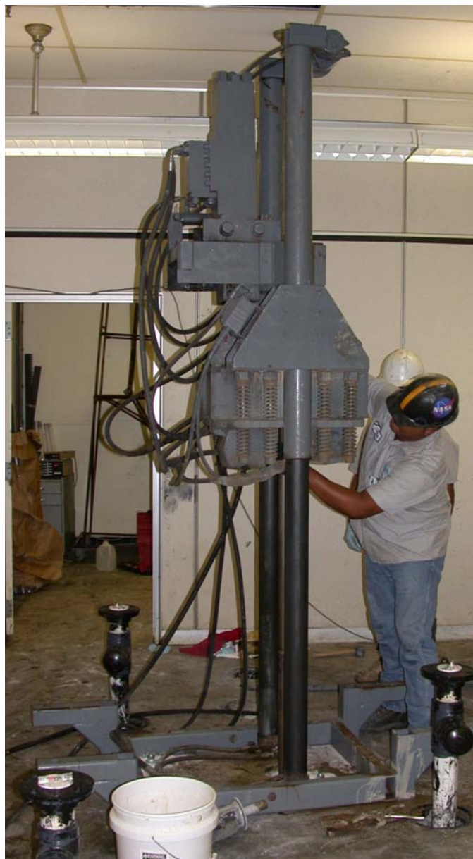
Figure 4-5. Indoor Vibra-Push™ Rig (LD Geoprobe® Series) Used in the EZVI Plot Inside the Engineering Support Building
