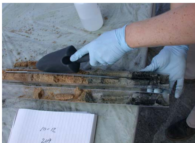
Figure 4-2. Soil Sample Collection (tan color indicates the native soil color; the gray to blackish band indicates evidence of the injected EZVI)
