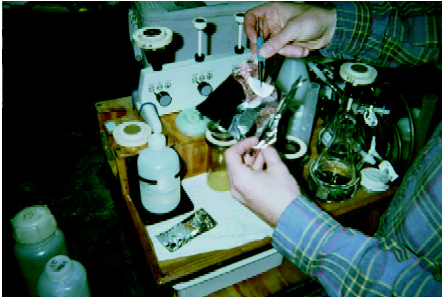
Figure 3.5 GF/F Filter Being Placed in a Foil Pouch
