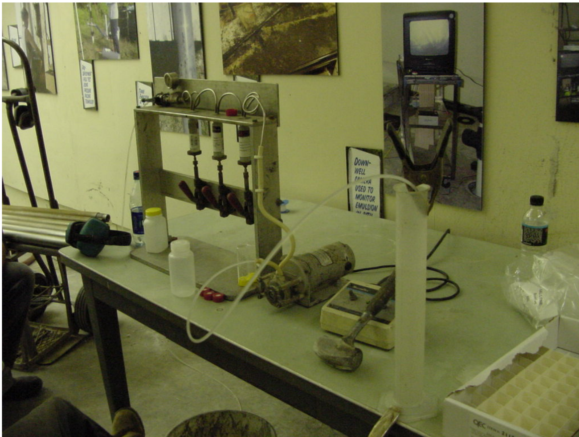
Figure 4-6. Collecting and Processing Groundwater Samples Using the Waterloo Profiler®
