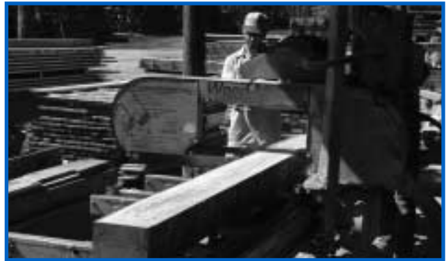
Resawing longleaf pine for flooring. The low moisture content (9% to 12%) of most reclaimed timber makes it ideal for remanufacture into flooring, molding, and other indoor building products.
