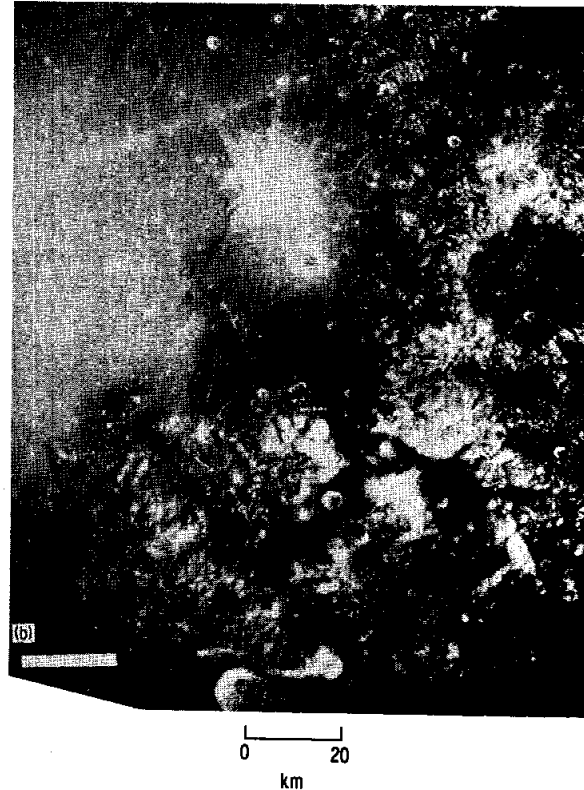
FIGURE 33-5.—Correlation of echoes to topography in the Taurus-Littrow area. (a) Generalized contour map of depolarized radar echoes in the Taurus-Littrow area near Apollo 17 landing site. (b) Topography of Taurus-Littrow area near Apollo 17 landing site (Apollo 15 metric camera frame AS15-0972). Area of photograph is same as that of part (a).
