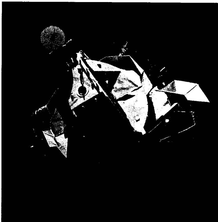
FIGURE 4-54.—The LM ascent stage pictured while stationkeeping with the CSM on revolution 52. The rendezvous radar antenna at the top of the LM is pointing at the CSM. The bell of the ascent propulsion engine is visible at the bottom of the spacecraft and, above it, the square hatch through which the crew egressed to the lunar surface. Above and to the viewer's right of the hatch, the commander's head is in sunlight in the triangular window. After docking and transfer of the crew and equipment to the CM, the LM ascent stage impacted into the lunar surface near the Apollo 17 ALSEP to provide a data point for the seismometer (AS17-149-22859).
