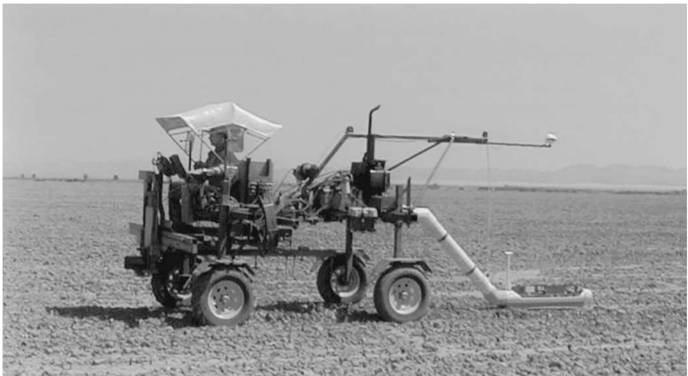
Fig. 10. Mobile dual-dipole electromagnetic induction equipment for the continuous measurement of apparent soil electrical conductivity.
