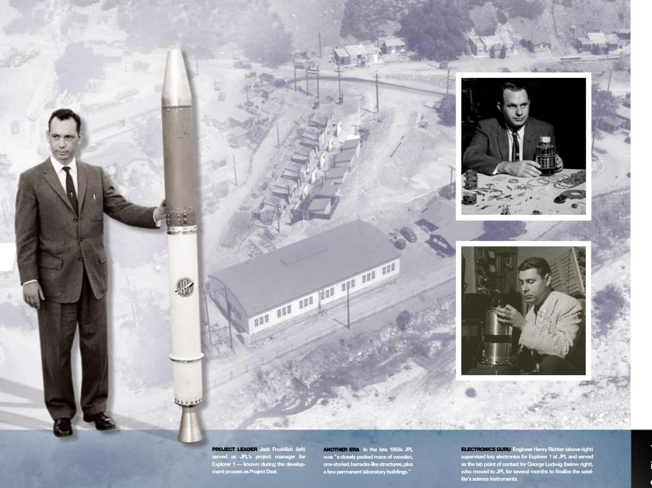
Perhaps the plum job was designing the satellite itself. The team rejected going with a sphere shape like the Vanguard satellite. The Jupiter C's upper stages sat on a rotating carousel that was spun up to 750 rpm — more than a dozen rotations per second — just before launch in order to stabilize the flight path. The bullet-shaped design was much like the concept sketched out by von Braun's engineer Boehm at Huntsville.
