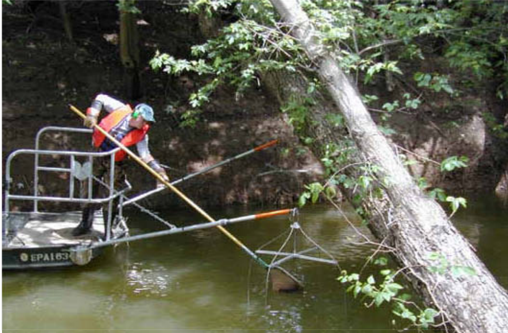
FIGURE 7-2. Net retrieval of fish stunned by boom-shockers, an active method.
