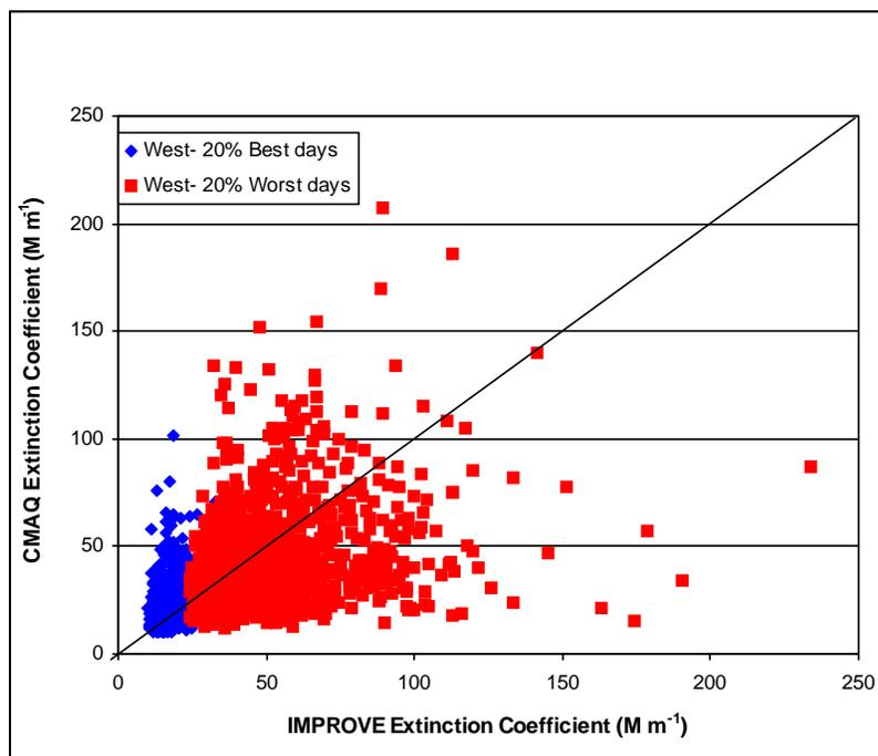
**Figure 53.** IMPROVE observed versus CMAQ predicted light extinction coefficient values on the 20% best and worst days in the West.
