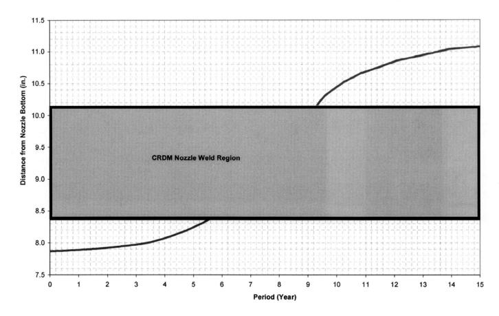
Figure 2: Through-Wall Axial Flaws Located in the 42.6 Degree Row of Penetrations, Uphill Side - Crack Growth Predictions (From Figure 6-19, WCAP-16027-P)
