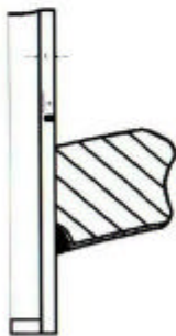
Figure D-10 Outside, Circumferential Surface Flaws, Along the Top of the Attachment Weld - Crack Growth Predictions (MRP Factor of 2.0 Included)
