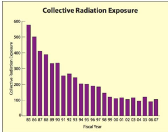
**Collective Radiation Exposure** - Total radiation dose accumulated by nuclear plant workers has decreased to less than 20 percent of the doses in 1985. In 2007, those workers receiving a measurable dose of radiation received about 0.1 rem (rem is a unit that measures the amount of radiation absorbed by the human body). For comparison purposes, the average U.S. citizen receives 0.3 rem of radiation each year from natural sources in the environment.
