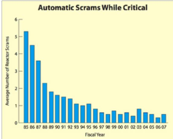
**Automatic Scrams While Critical** - A nuclear plant is designed to automatically shut down (scram) if a safety problem is detected while operating. This chart shows the average number of scrams has decreased dramatically over the past 20 years, indicating far fewer safety problems in plant operations. In FY 2007, there were about 50 unplanned scrams among 104 operating plants compared to over 500 scrams in 1985.
