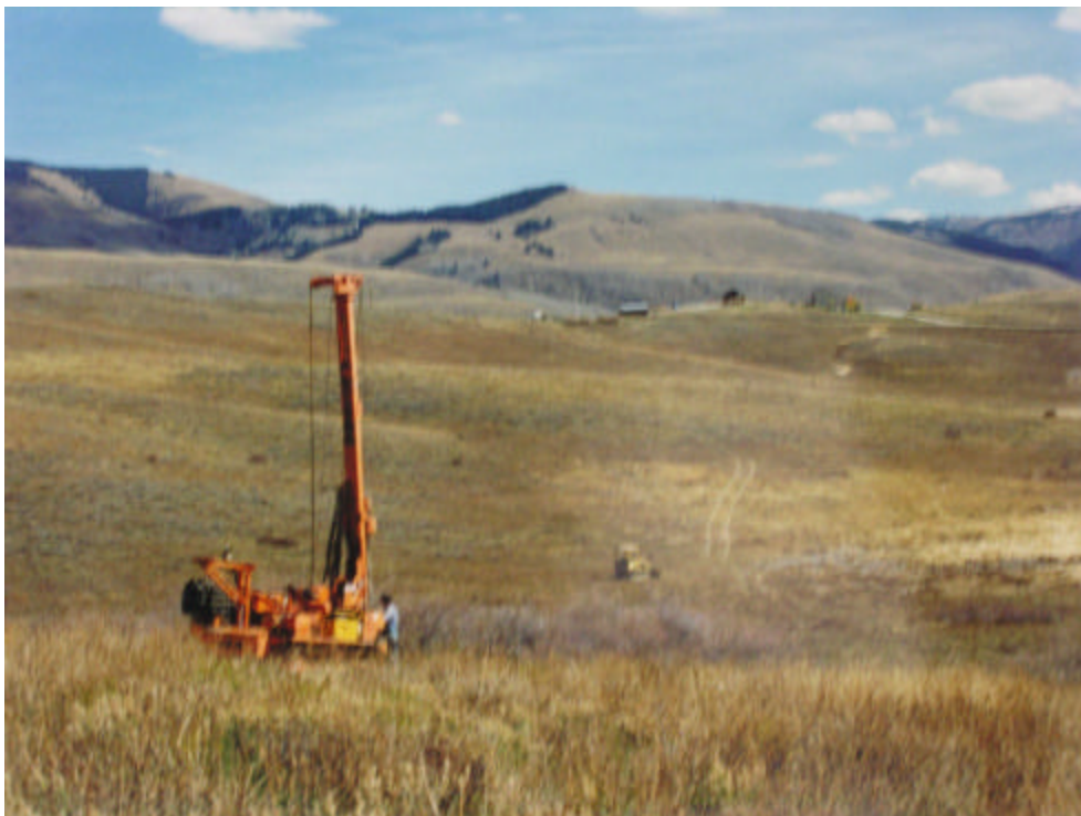
Fig. 3. Acker rig drilling hole #5 in 1994, at toe of East Slide. Note equipment's tracks in grass at right center.
