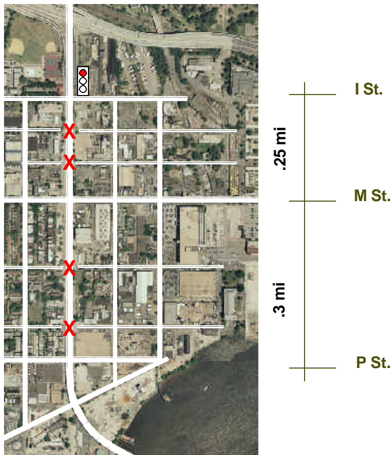
Crossing analysis of existing conditions; x indicates no current continuity across South Capitol Street
