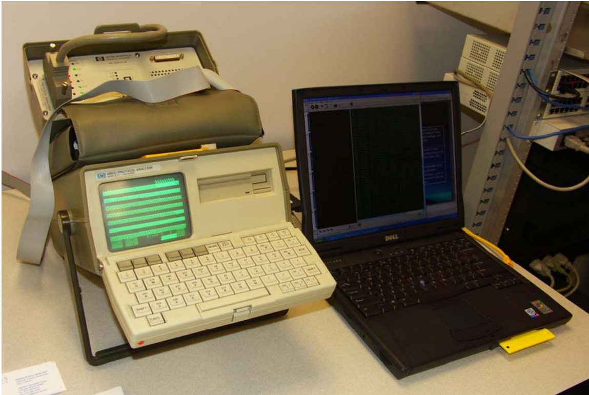
Figure 18. Network Analyzer and Notebook Computer Used To Measure Performance
