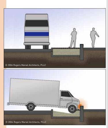
A vehicle can be immobilized by the collapsible material of the Tiger Trap™ system.
