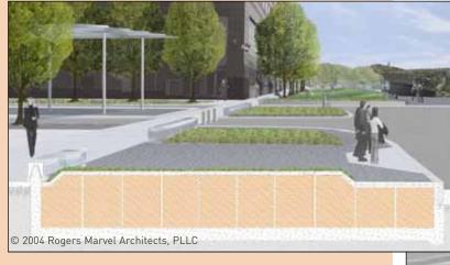
The Tiger Trap™ system can protect against a vehicle attack without impeding open public spaces.
