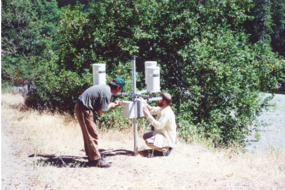
Figure 3.2.2. Installation of a three tipping bucket rain gauge cluster, with dual data loggers, at Legget, CA.
