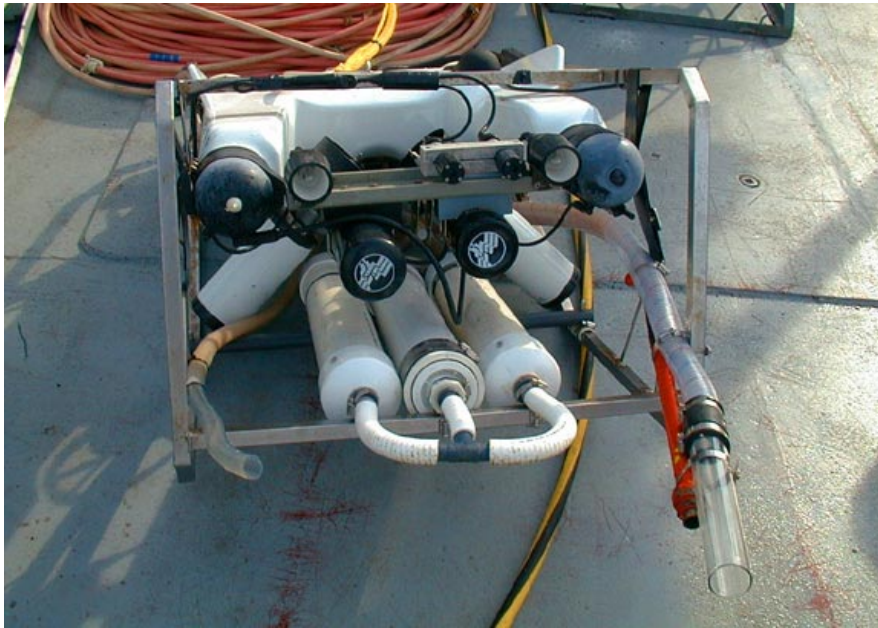
Remote Operating Vehicle (ROV) equipped with suction sampler, provided by the National Undersea Research Center at UNC-Wilmington.
